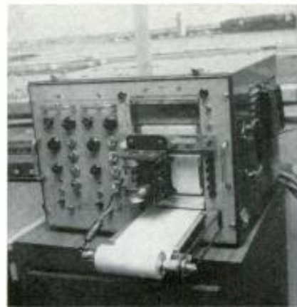
Figure 6. The graphic-level recorder used to preserve the aircraft sound measurements.
