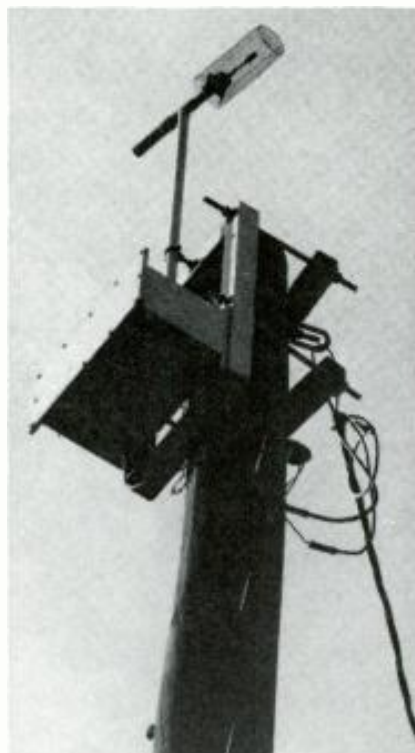
Figure 5. This close-up of a remote monitor station such as in Figure 2 shows the microphone to be parallel to the ground so that sound impinged on it in a grazing fashion.
